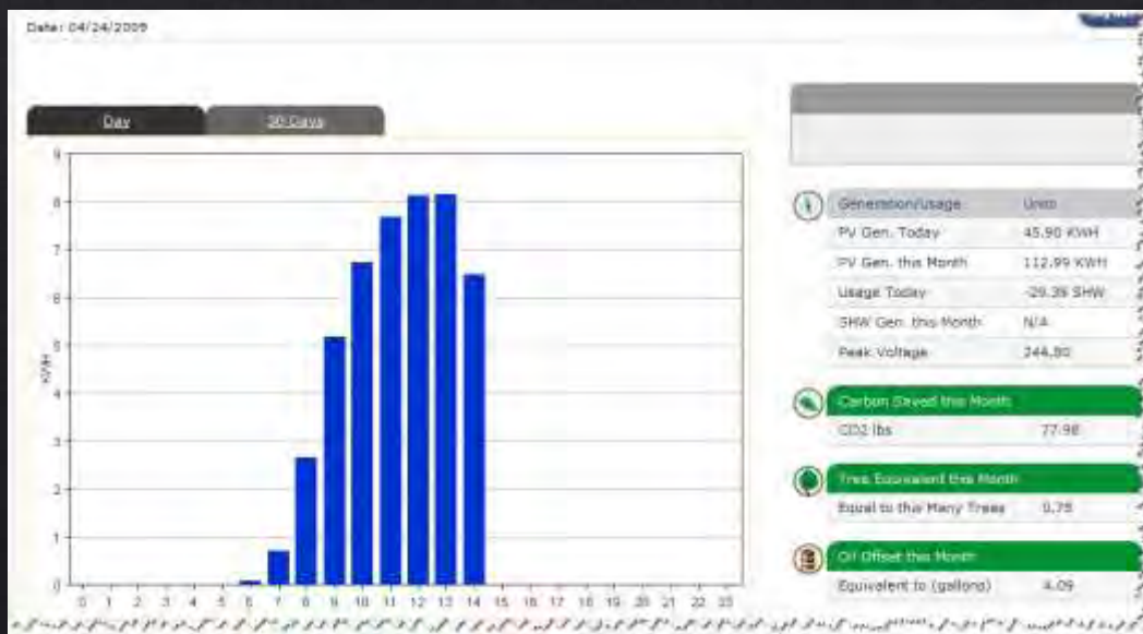
Web-based home power monitoring system
