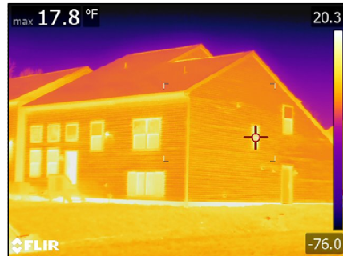
With Exterior Insulation
