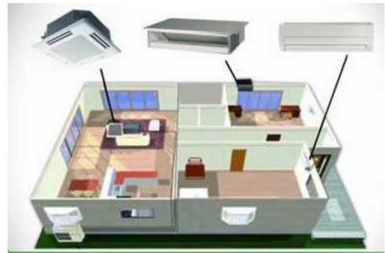
Split system heat pump
